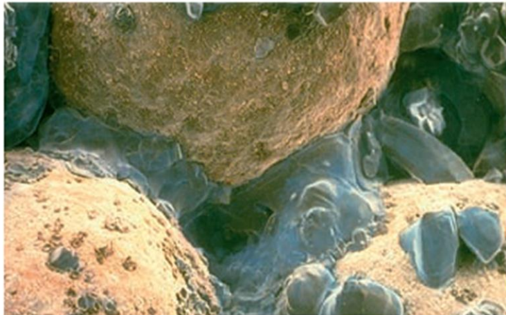
Crystal bridges between fertilizer particles cause caking
